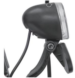
5.2 Adjust the headlight to a proper angle by this way: loosen the adjusting bolt with a cross-head screwdriver, adjust the headlight tilt angle to the best position, and then tighten the bolt.
