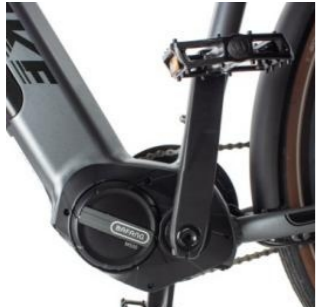
Left pedal tightens counter clockwise
